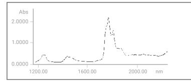
These two scans demonstrate the effect of varying the SBW. The above graph shows a scan of hexane with a SBW of 15 nm.
